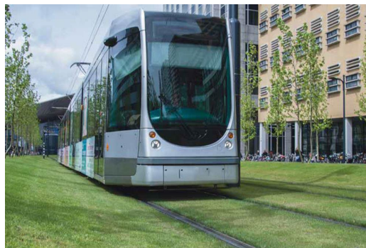
Plinth with rail boot only – Vegetation at top of rail *ABI's preference
